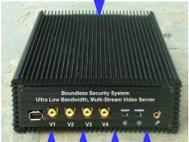
It provides an internal Network Video Recorder for continuous recording of its, and others', many IP-video streams.
